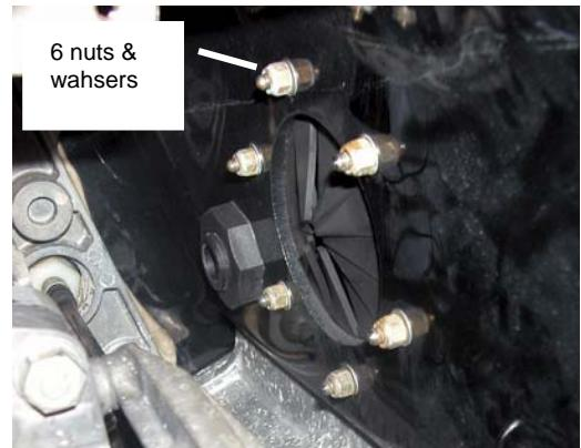
Remove OEM exhaust outlet hose from inside of hull. Remove aluminum ring with studs from exhaust outlet hose. **Retain ring.** Discard exhaust outlet hose and exhaust outlet valve.
