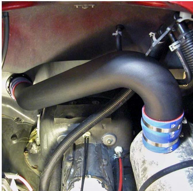
Tighten hose clamps (2) securing Exhaust Tube in place. **NOTE: Do not over tighten clamps.** Tighten coupler securing exhaust pipe to water box inlet if loosened.
