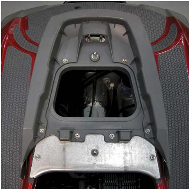
Inside engine compartment at rear of craft remove and discard exhaust baffles<sup>1</sup> and hose<sup>2</sup> between water box and exhaust outlet hose. **Save OEM clamps for installation portion.**
